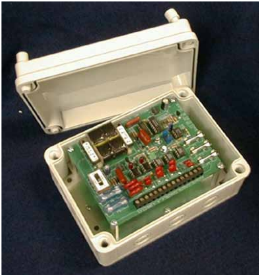
Optional Sentry 50 Vynckier enclosure 7" x 5" x 3" (or 7" x 7" x 3") UV Stable Polycarbonate
